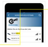
Find visible devices and select the NORDAC ACCESS BT (TIE5-BT-DE:12) The Status LED will flash blue quickly as soon as the modules have been scanned.
