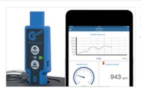
The dashboard opens, and the Status LED lights up blue. The NORDAC ACCESS BT is now connected with the terminal device.
